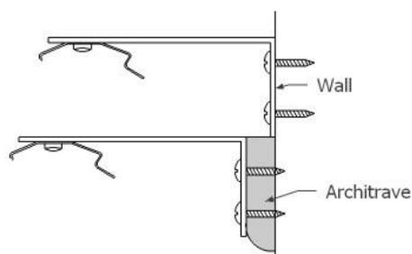
Alternate positions, depending on a solid fixing point (determined at the time of measuring, as it will affect blind size)
